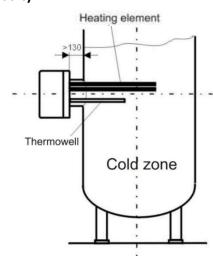
Too long flange welded too high. Thermowell under the heating element.
