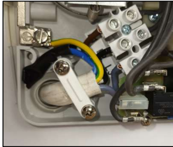
Connection example 3 x 400 V
