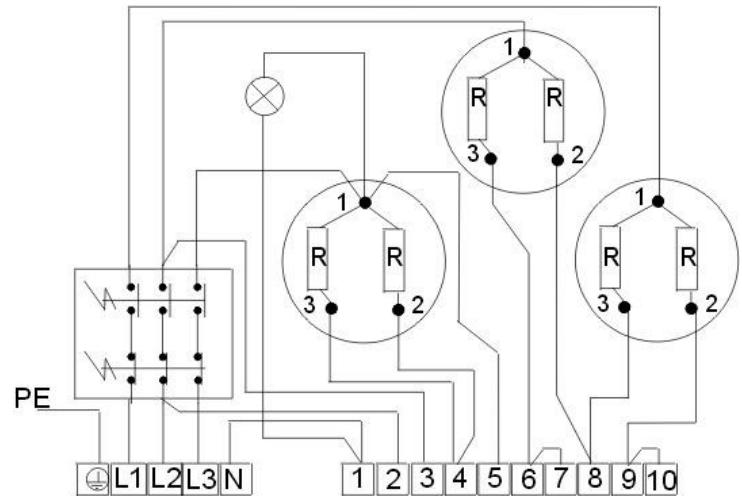
3 kW 1 PE - N AC 230 V / 50 Hz
